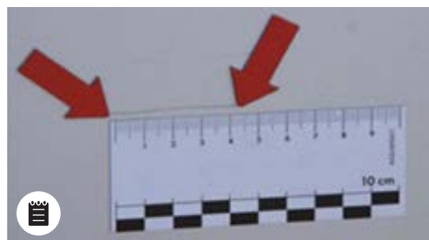
Polishable damage or scratch \leq 50 mm
