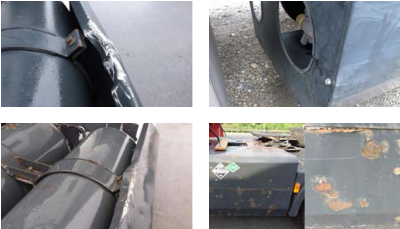
Visible dents and deformations that affect the functionality and/or safety → charge for replacement of protective covers. Rust, breakages and/or gouges that affect the functionality and/or safety → charge for replacement of protective covers. Where the covers are absent → charge for the replacement of these.
