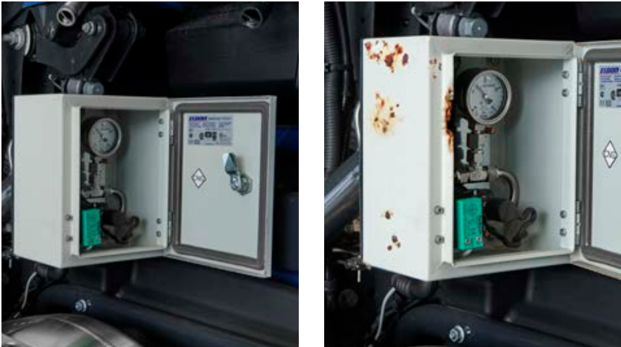
Rust on the fill receptacle protection box → note without charge for damage.
