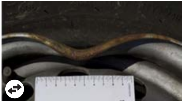
Rim lining damaged, non-compliant rim. Valuation of a dimensional check to check safe state of the vehicle
