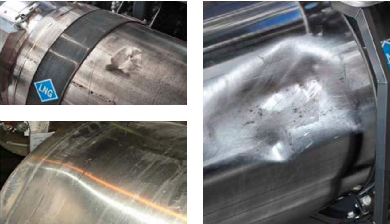
Evidence of tank repairs → charge for tank replacement.
