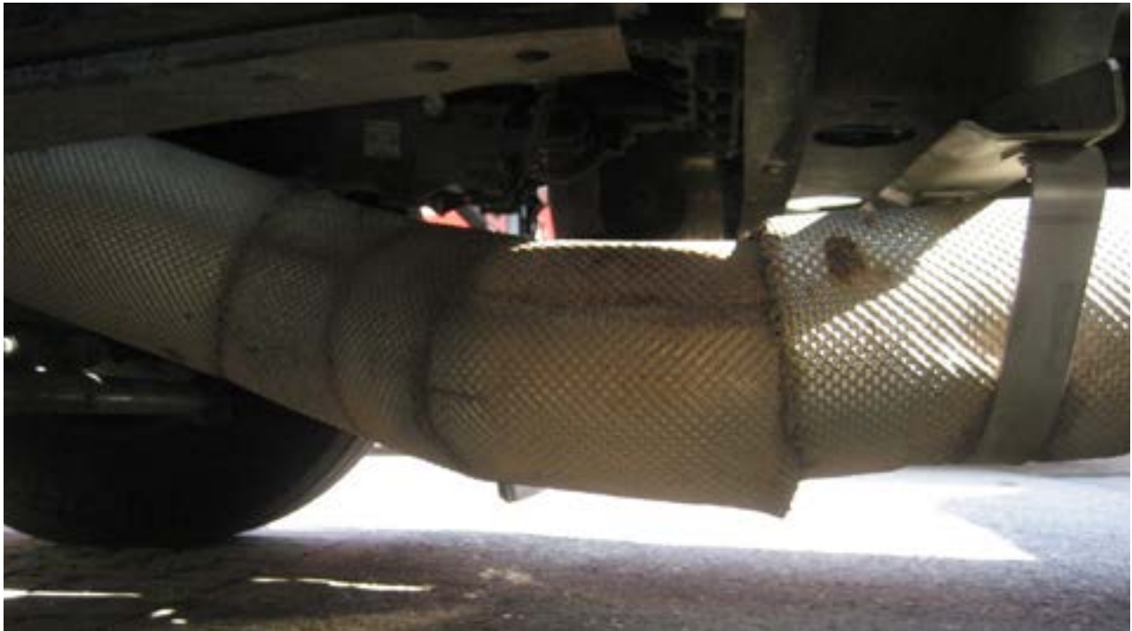
The following are not accepted: broken pipes, torn thermal insulation, scratches that are deep in the material, dents that reduce the pipe diameter.
