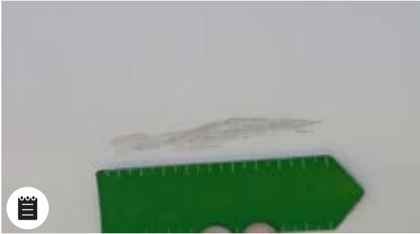
Side panels: Faint scratch with material removal ≤ 20 cm
