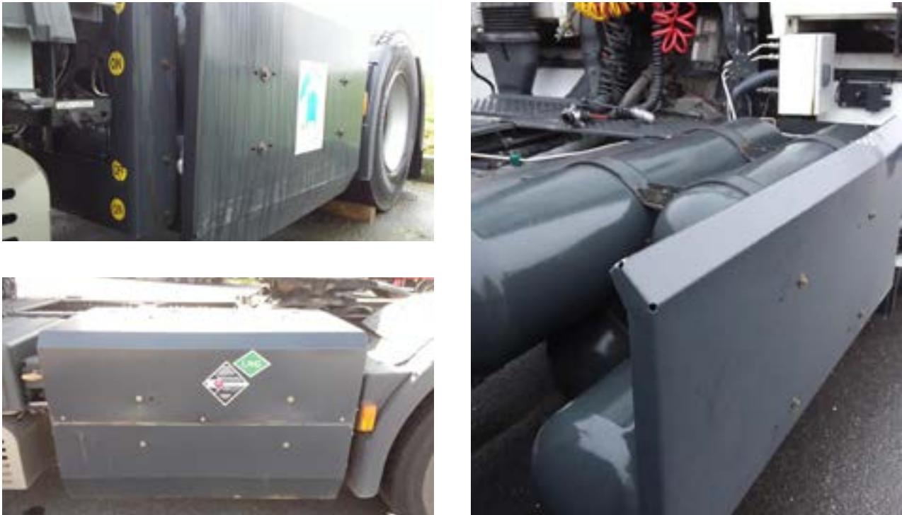
CNG cylinders must be returned in proper conditions as illustrated in pictures. Dents, deformations, rust and/or gouges that do not affect functionality and safety are accepted.
