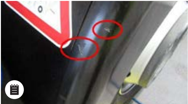
Scratches that cannot be felt with your nail and surface ≤ 45 cm² (equivalent to a credit card)
