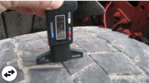
Tyres: Notch > 3 mm deep, removal
