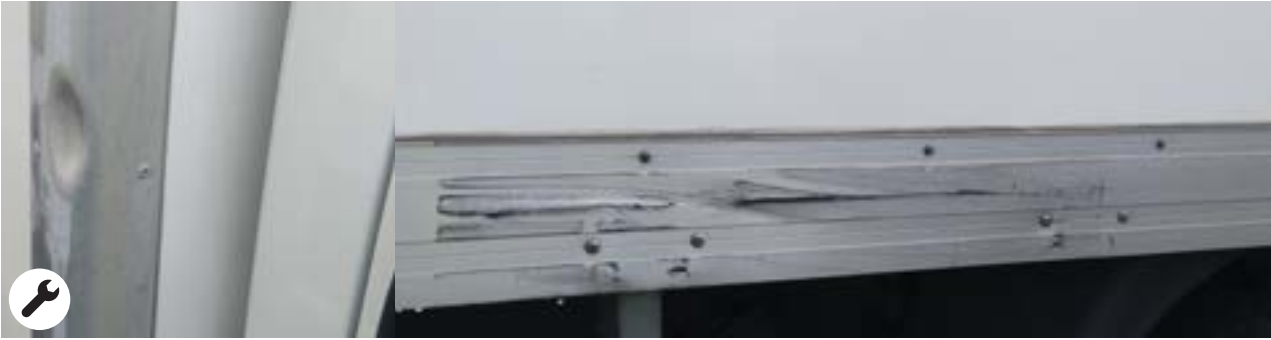
Underbody side profiles: Deformations within economic repair
