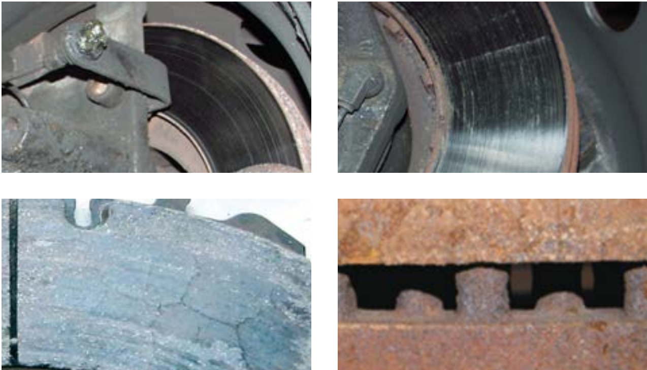
Normal condition and conforms to the age and mileage of the vehicle Brake pads thikness > 30 %
