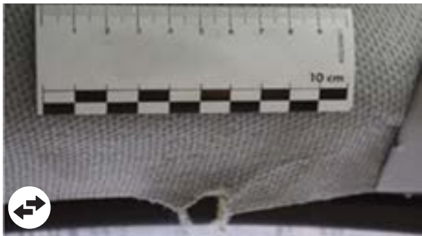
Fabric trim: Tear, hole > 5 mm, indelible marks
