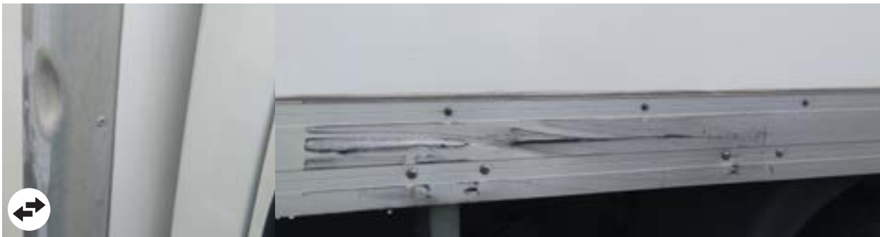
Underbody side profiles: Deformations > or = 10 cm
