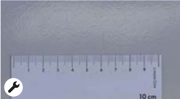
Repainted with fault (dimpled appearance). Paint too thick, insufficient, with inclusion of particles
