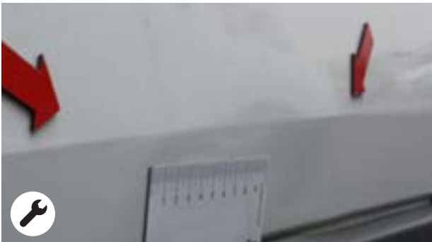
Defect: Deformed panel following repair
