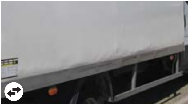
Fiberglass side panels: Deformation on lower part, length of > 1 m Notes: Replacement of the front panel of the underbody requires removal of the underbody.
