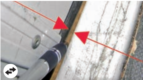
Deformations in the body closures if > or = 10 cm, closure not possible or not sand-proof
