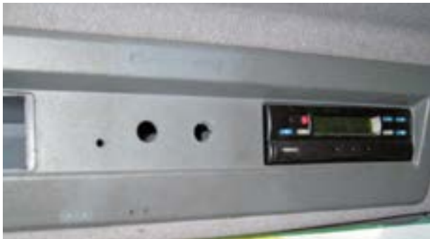
Control parts, seat or trim pieces missing, broken or pierced
