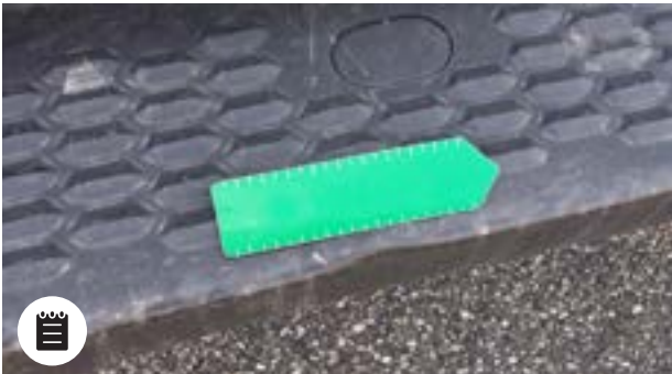
Rear Step Slight deformation if \leq 3 cm total length or cumulative (i.e. nbr 3 deformations of 1 cm each)
