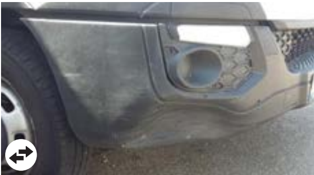
Broken, removal of material or deformation beyond economic repair or not feasible
