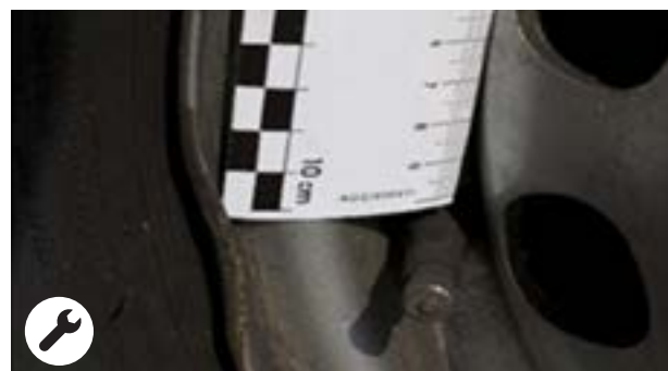
On steel rim: Attachment edge slightly deformed
