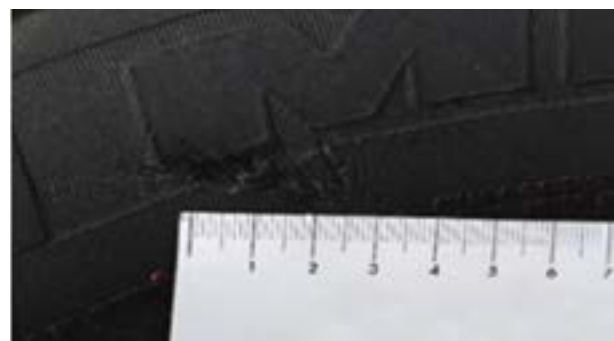
Tyres: Notch \leq 3 mm deep (CONFORMS)
