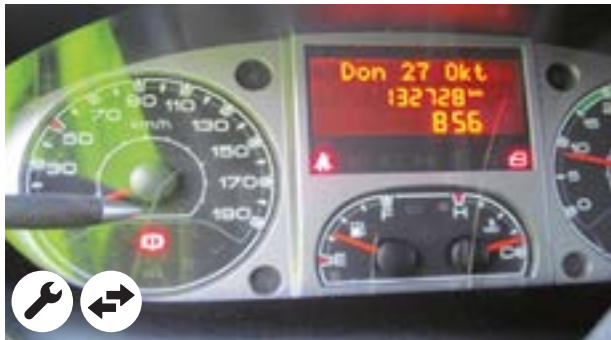
Scratches on the combined instrument panel and other visuals
