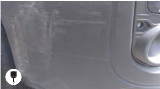
Scratches that can be felt with your nail and surface > 45 cm² (equivalent to a credit card)
