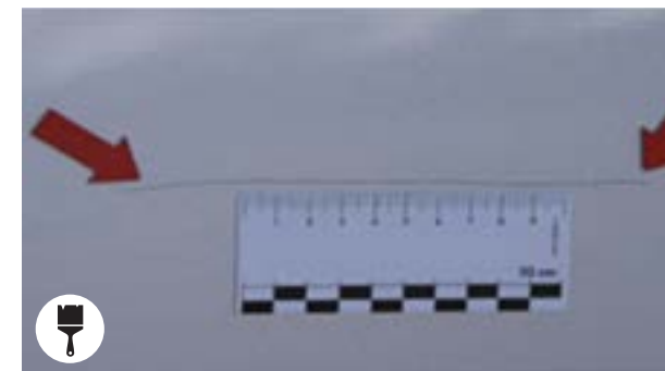
Scratches > 20 mm Note: On rear swinging door it is not possible to paint per half panel
