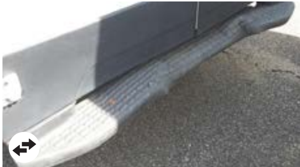
Rear footboards: Deformations > 3 cm
