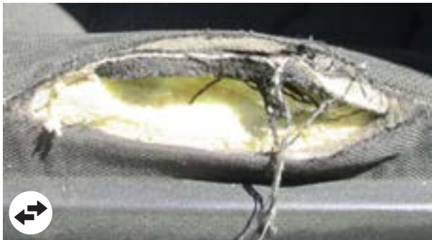
Foam missing or broken frame
