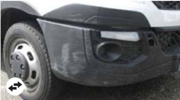
Removal of material or deformation feasible or economical to repair if > or = 10 cm
