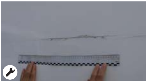
Side panels: Scratch with removal of material \geq 10 cm within economic repair. Option to paint half panel
