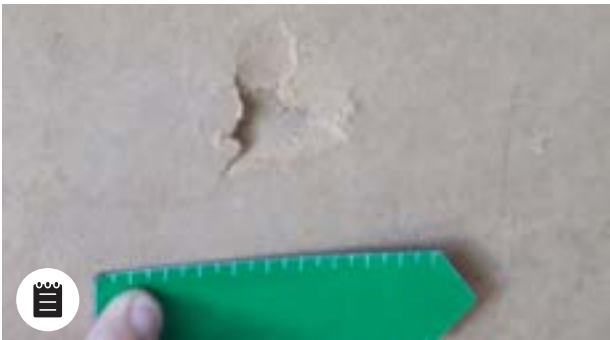
Wood internal protections: Small impacts \leq 2 cm
