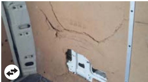
Wood internal protections: Impacts > 2 cm, torn panel, panel missing (excluding door upper panels)
