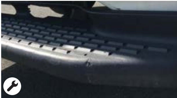
Rear footboards: Deformations within economic repair
