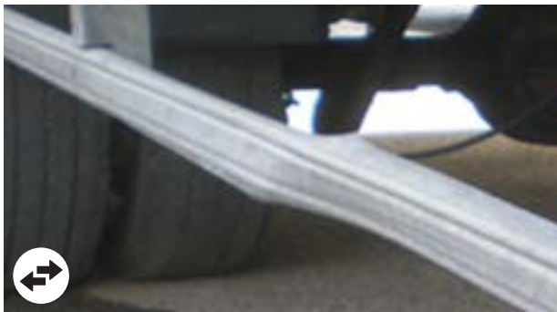
Side underun guards: Deformation beyond economic repair
