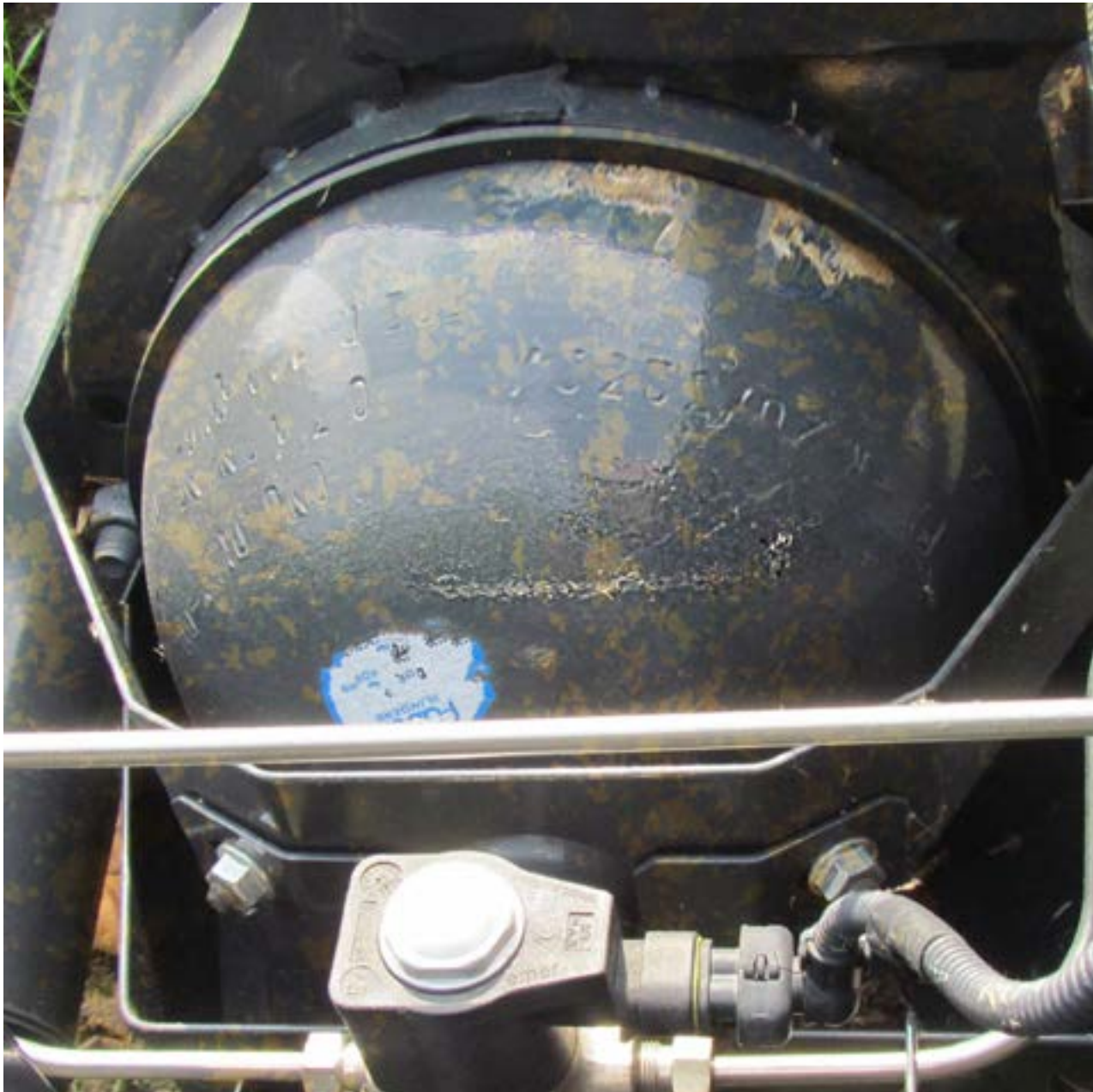
Original CNG cylinder identification markings absent or illegible charge for replacement of CNG tank with a new one
