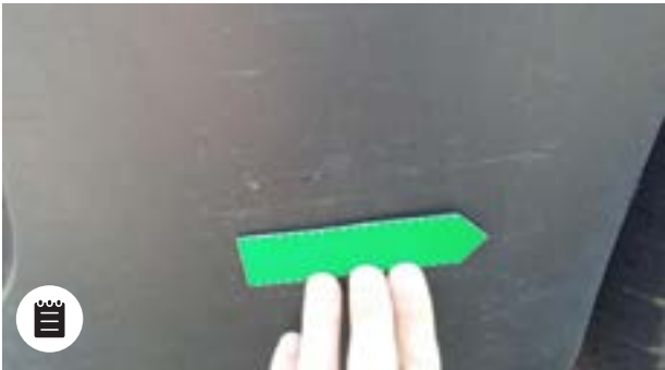
Scratches that can be felt with your nail or surface ≤ 45 cm² (equivalent to a credit card)
