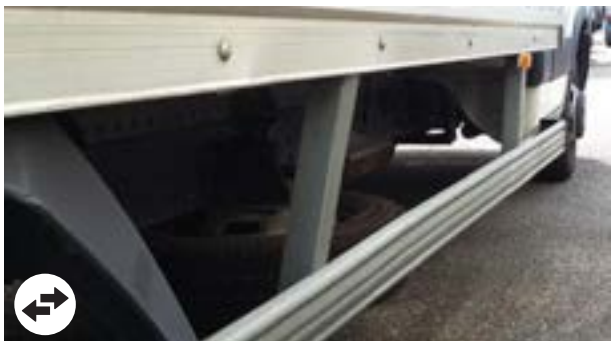
Side underun guards: Deformation within economic repair
