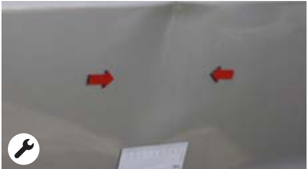
Indentations > 20 mm in diameter; altered paint, hail damage or significant pockmarks Notes: Smart repair possible on isolated, significant pockmarks if paint is not altered
