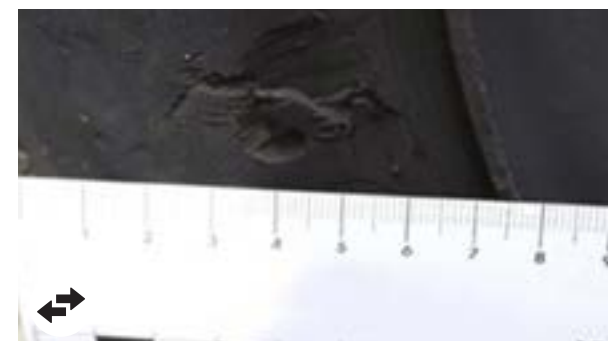
Tyres: Notch > 3 mm deep, removal
