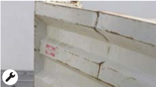
Deformations in the body closures with a repair time > 1 h within economic repair and if < di 10 cm
