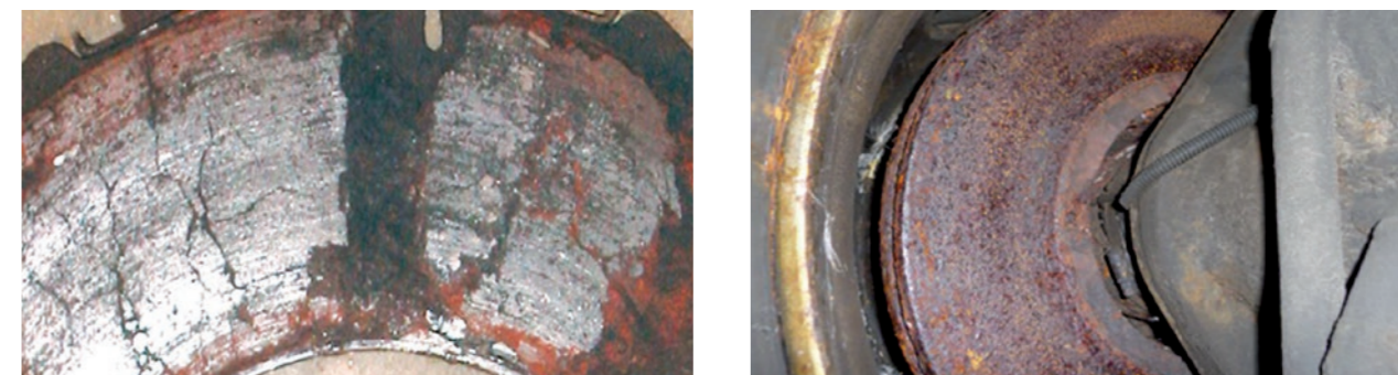
Rusted, ground, worn brake discs
