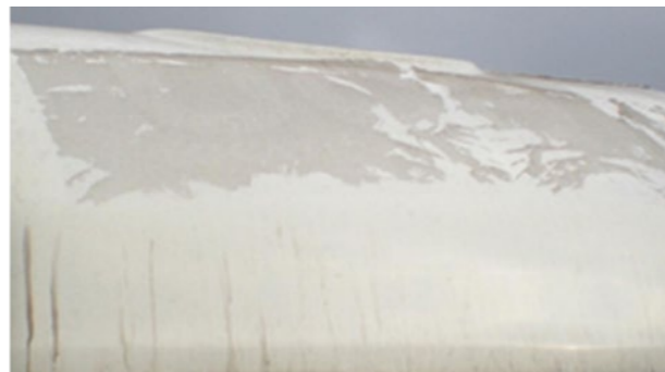
Trace of glue. NB: Presence of tags or graffiti, valuation in real time during cleaning and/or buffing
