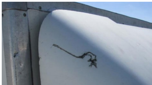
Cabover and deflector: Within economic repair
