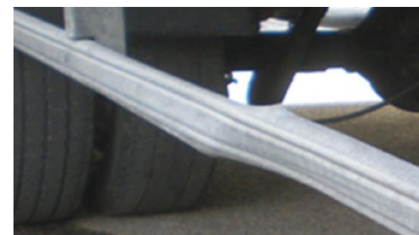
Side underun guards: Deformation beyond economic repair
