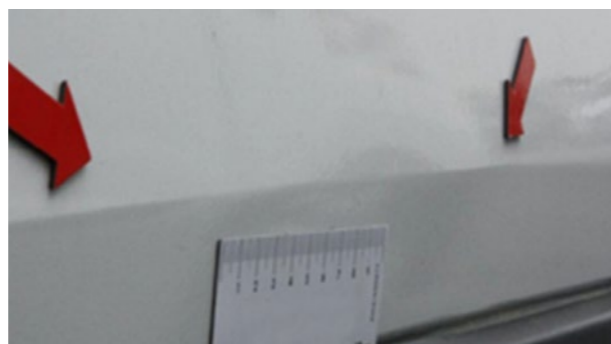
Defect: Deformed panel following repair
