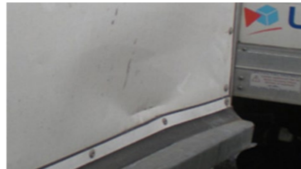
🔧 Side and rear doors: Significant deformation: Repair time > 1 h within economic repair; closure not sealed
