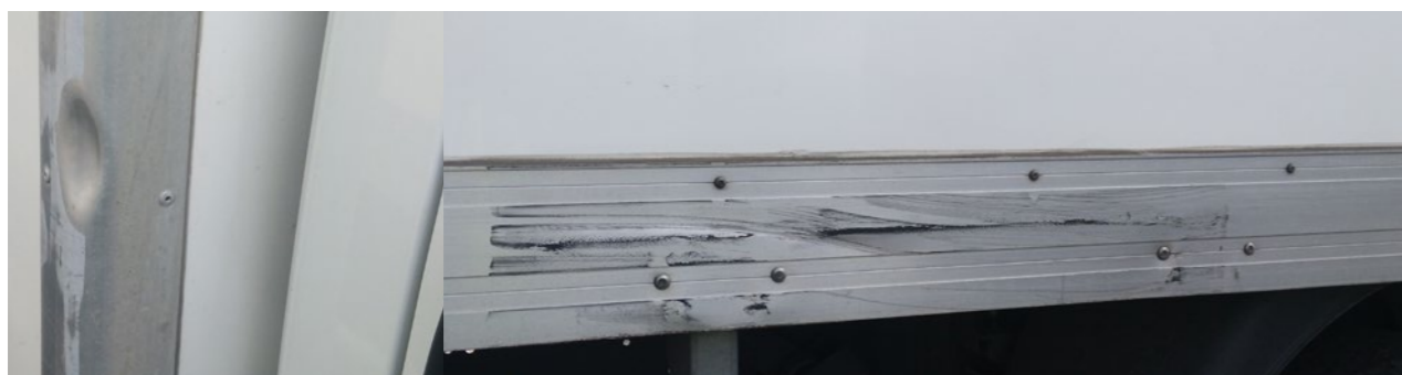
Underbody side profiles: Deformations within economic repair
