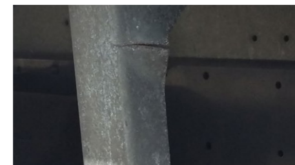
Tail lift: Deformations of platform within economic repair
