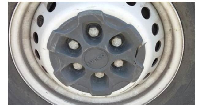
Wheel covers: Deformed, broken, material missing or removed
