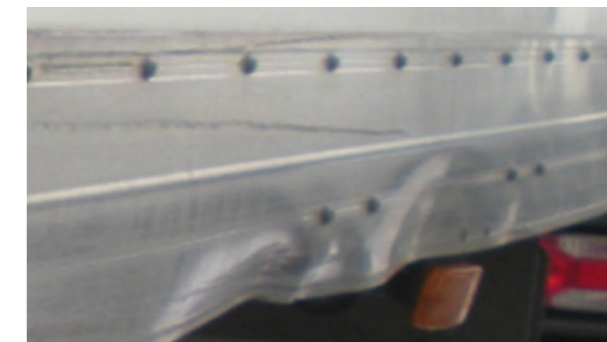
Underbody side profiles: Deformations beyond economic repair, perforations, removal of a section of the profile
