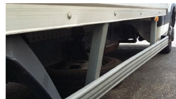
Side underun guards: Deformation within economic repair
