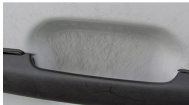
Faint superficial scratches, e.g. at the fuel filler cap, hatches, door handles, bumpers and trims
