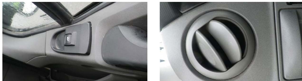
Slight decolouration due to sun exposure
